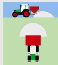
**DISC TYPE SPREADER PATTERN:** Material is subjected to wind influence. The flat pattern requires precise overlap.
