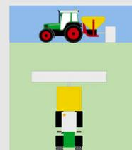
**PENDULUM SPREADER PATTERN:** Wind influence is negligible. Tractor does not get covered with fertilizer.
