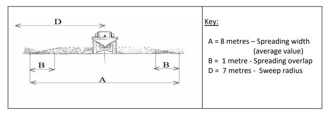
The operator must close the hopper exit slots during transfers, along field edges and each time he completes a sweep.
