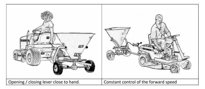
! For safety reasons no persons or animals must be within a 10 meters radius of the fertilizer spreader during spreading operations.
